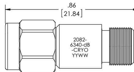
Table with 4 columns: QTY., PART NUMBER, DESCRIPTION, ITEM NO. Row 1: X, 2082-6340-dB-CRYO, ATTENUATOR, SMA-m/f, DC-18 GHz, 2 WATTS AVG, 500 WATTS PEAK. Row 2: 1, TA-2082-6340-dBU, ASSEMBLY, ATTENUATOR, SMA-m/f, DC-18 GHz, 2 WATTS AVG, 500 WATTS PEAK, UNMARKED, 1
